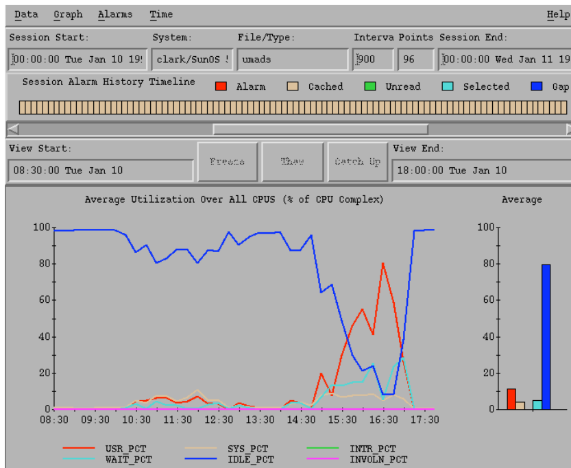
(b) UMA tool (MAP) showing processor utilization as a time series and as a histogram. A sliding control enables seamless transition between both monitored and historical data.
